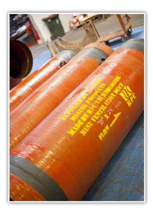
RPC Technologies is the manufacturer and supplier of GRP Mine Ventilation Duct (MVD).
